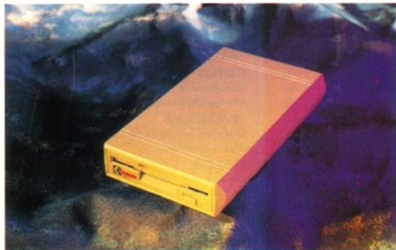
The Cumana drive has curiously sloping sides, so it can't stand on its edge. The case also seems rather thin in places.
